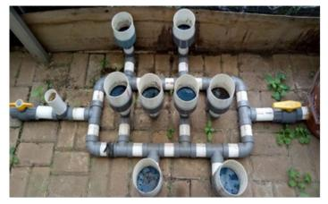
Figure 4 Prototype of the Irrigation system
