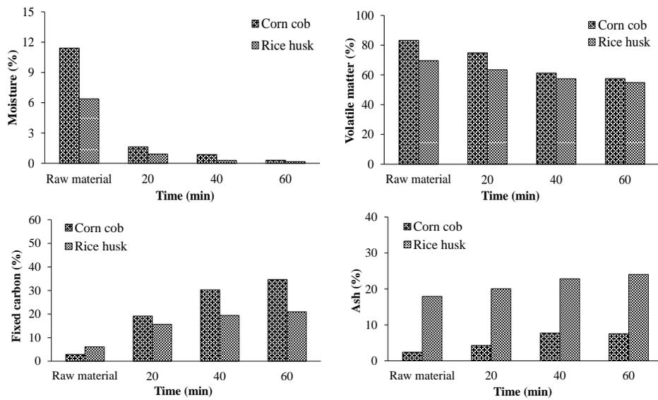
Figure 4 Effect of residence time on proximate properties at 300 °C of torrefaction temperature
