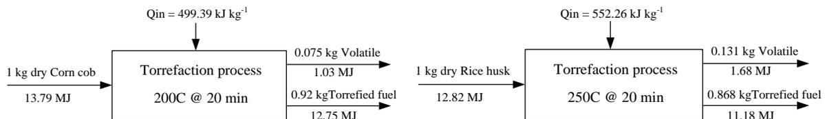
Figure 10 Energy balance diagrams
