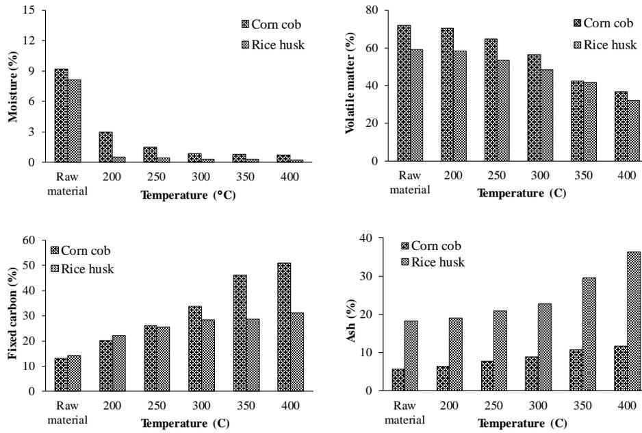
Figure 3 Effect of torrefaction temperature on proximate properties at 40 min of residence time
