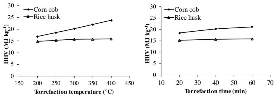
Figure 7 The effect of torrefaction temperature and time on heating value
