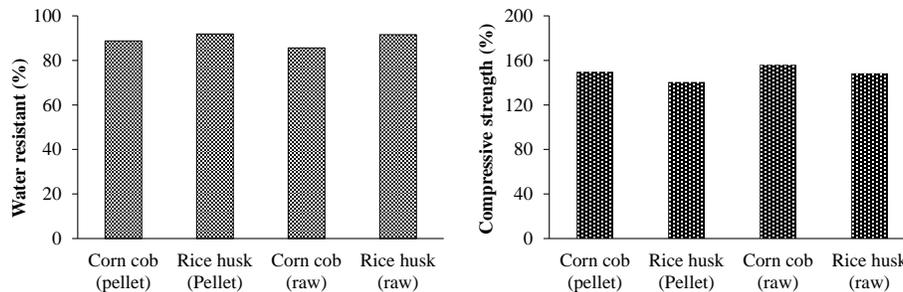
Figure 9 Water resistance and compressive strength of torrefied and raw pellet fuels
