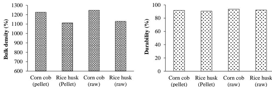
Figure 8 The bulk density and durability of torrefied and raw pellet fuels
