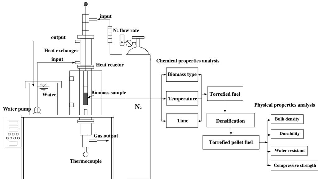
Figure 2 Schematic diagram of the torrefaction experiment for pellet fuels
