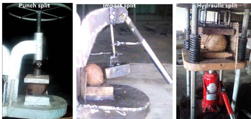
Figure 1. Experimental cracking devices
