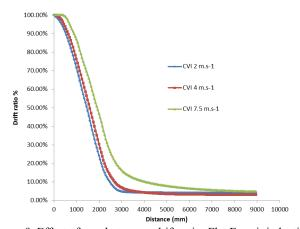
Figure 9 Effect of nozzle type on drift ratio- Flat Fan air induction nozzle (CVI single jet)
