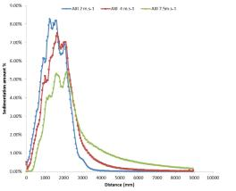
Figure 5 Deposition amount at different wind velocities using Flat
