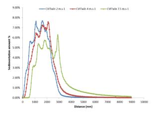
Figure 7 Deposition amount at different wind speeds using Flat Fan nozzle air induction Twin jet (CVITwin)
