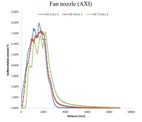
Figure 6 Deposition amount at different wind speeds using Flat Fan nozzle air induction single jet (CVI)
