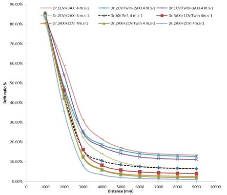
Figure 12 Effect of nozzle substitution on drift ratio at 4 m s<sup>-1</sup> wind speed compared to the reference nozzle
