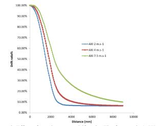
Figure 8 Effect of nozzle type on drift ratio- Flat fan nozzle (AXI)
