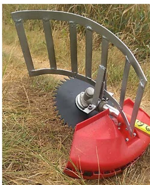
(b) Metal guard attached to the gear head
