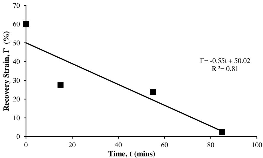
Figure 7 Recovery strain  $\Gamma$  against time after load removal
