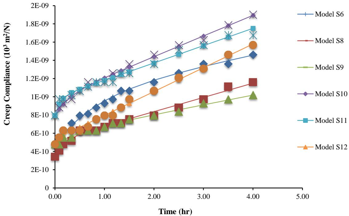
Figure 5 Comparison between the experimental data (EXP Sn) and the generated estimate of the Burgers model (Model Sn) against time for day 1 samples
