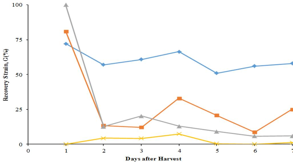
Figure 9 Interaction graph of recovery strain  $\Gamma$  against days after harvest at different test times (T1 is 15 minutes after load removal, T2 is 20 minutes after load removal, T3 is 60 minutes after load removal and T4 is 90 minutes after load removal.)
