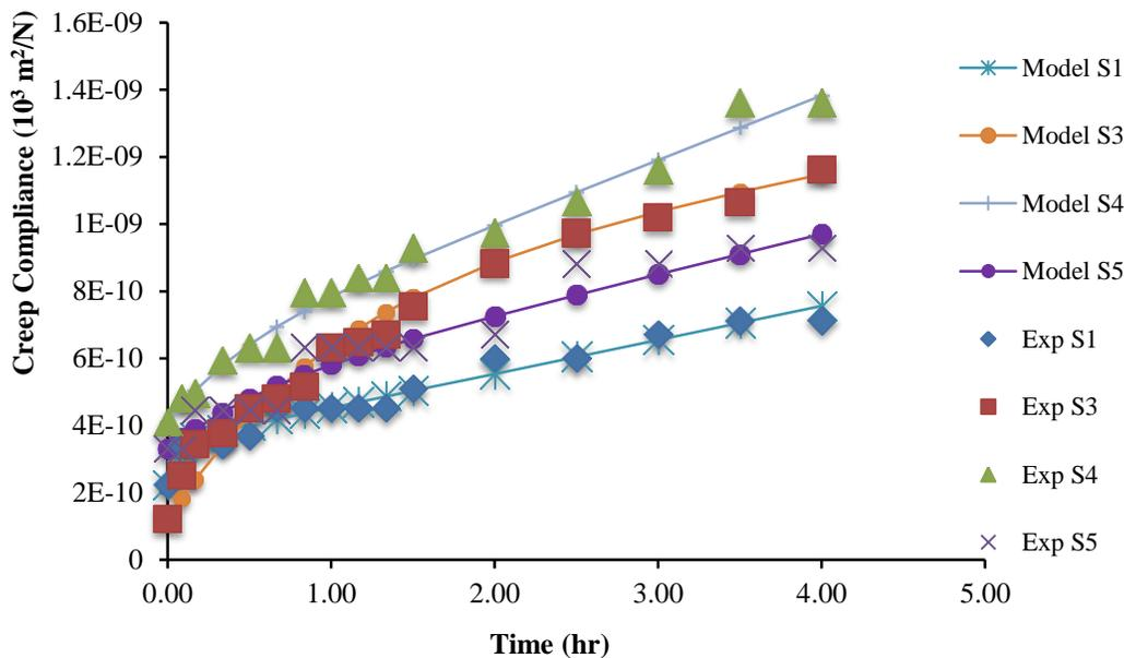
Figure 4 Comparison between the experimental data (EXP Sn) and the generated estimate of the Burgers model (Model Sn) against time for day 1 samples
