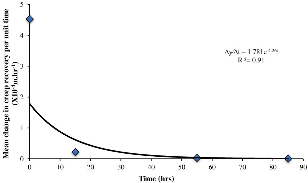
Figure 6 Rate of change in creep recovery against time after load removal
