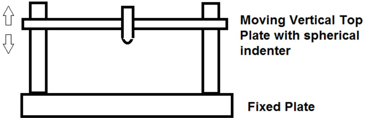
Figure 1 Constant load tester
