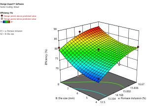
Figure 2 Three-dimension graph for machine efficiency over the pomace inclusion and die size
