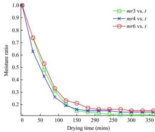
Figure 1 Moisture ratio against time at microwave power of 90 W
