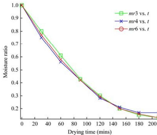
Figure 2 Moisture ratio against time at microwave power of 100 W
