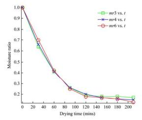
Figure 3 Moisture ratio against time at microwave power of 120 W
