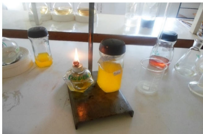
Figure 5 Fueling lamp test of biodiesel of C. megalocarpus
