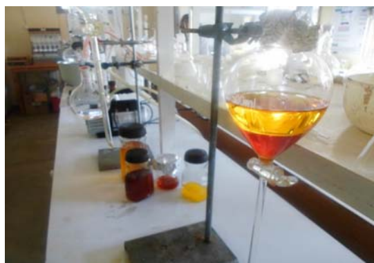
Figure 3 Biodiesel separation from glycerol (right side)
