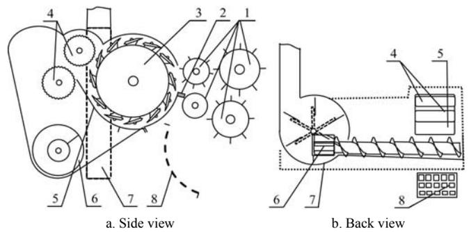
Figure 4 The cylinder type chopper of a forage harvester with a blower
