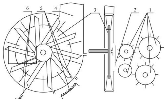
Figure 6 A chopper system with a flywheel cut and throw cutterhead
