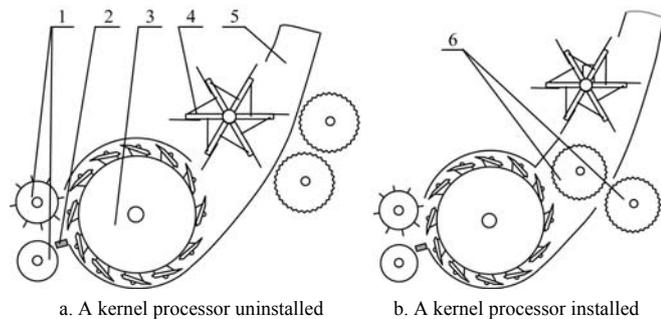
Figure 1 Precision cut chopping system with a cylinder cutterhead and a crop accelerator of a self propelled forage harvester
