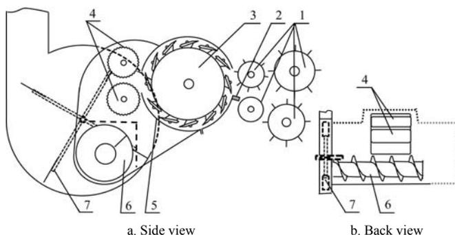
Figure 3 The cylinder type chopper of a forage harvester with a blower
