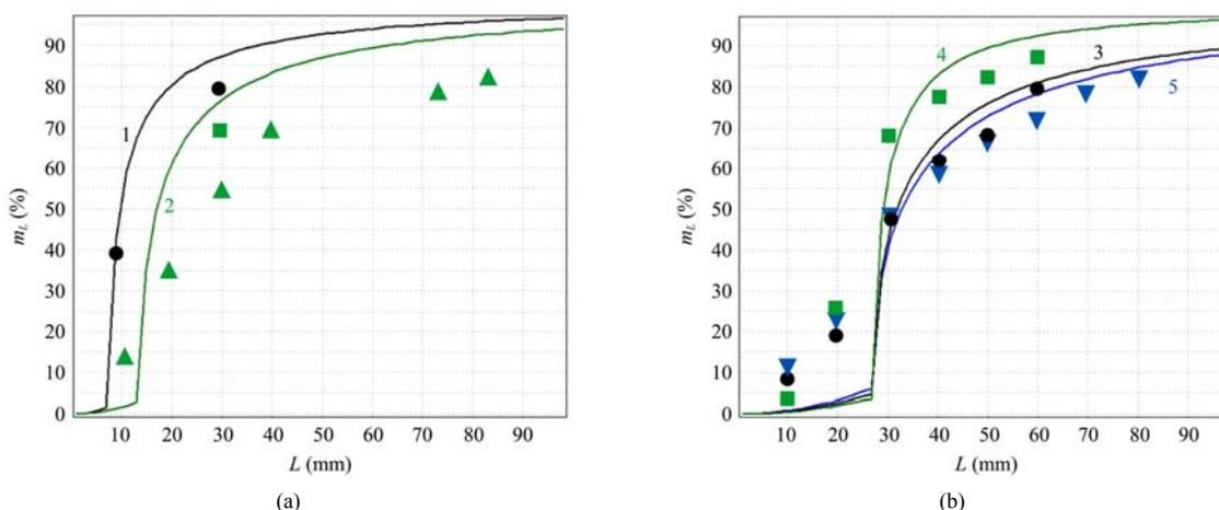
Figure 8 Effect of  $L$  on  $m_L$  with results of field tests of forage harvesters KSK-100 and KPU-75 on chopping cereals for haylage (a) and results of laboratory tests of a chopper of forage harvester KSK-100 (b)
