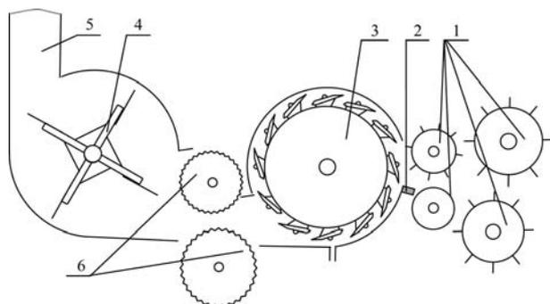
Figure 2 Precision cut chopping system of a trailed forage harvester
