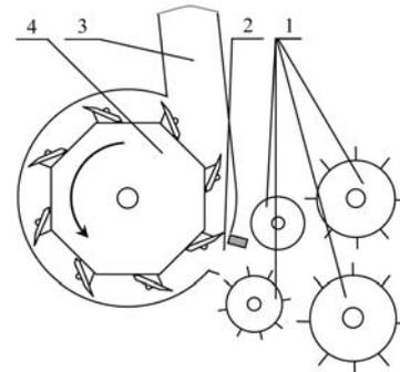
Figure 5 A chopper system with a cylinder cut and throw cutterhead
