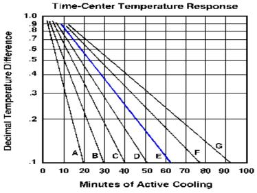
**Figure 1.** Time-temperature response of various fruits and vegetables immersed in agitated chilled water at 1.7°C (Boyette et al. 1992).
