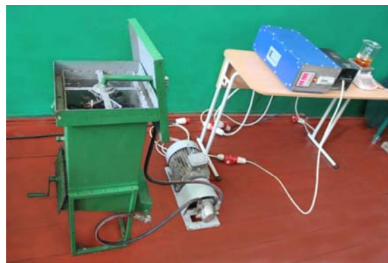
Figure 3 Pilot sample of the hydro-mechanical mixer for the diesel biofuel production
