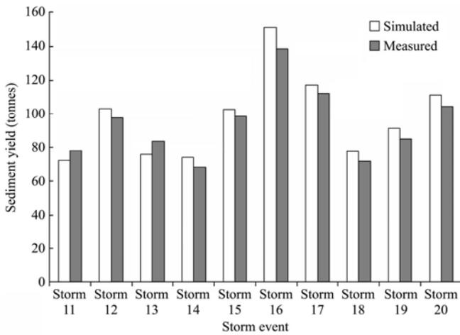
Figure 6 Comparison of the predicted and measured sediment yield for 10 storm events
