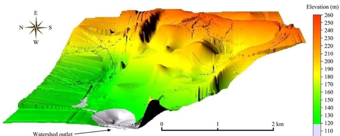
Figure 5 Digital Terrain Model of Ofuloko Watershed
