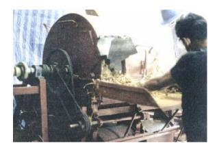
Figure1: Testing of developed soybean threshing unit
