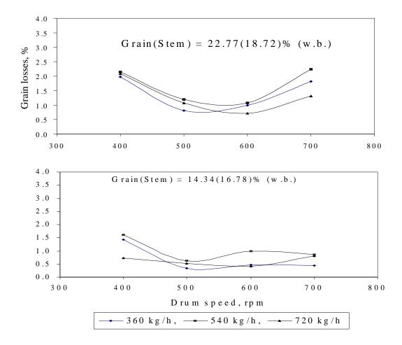
Figure 5: Effect of drum speed on grain losses at different grain moisture contents and feed rates.
