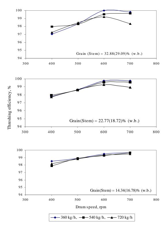
Figure 4: Effect of drum speed on threshing efficiency at different grain moisture contents and feed rates.
