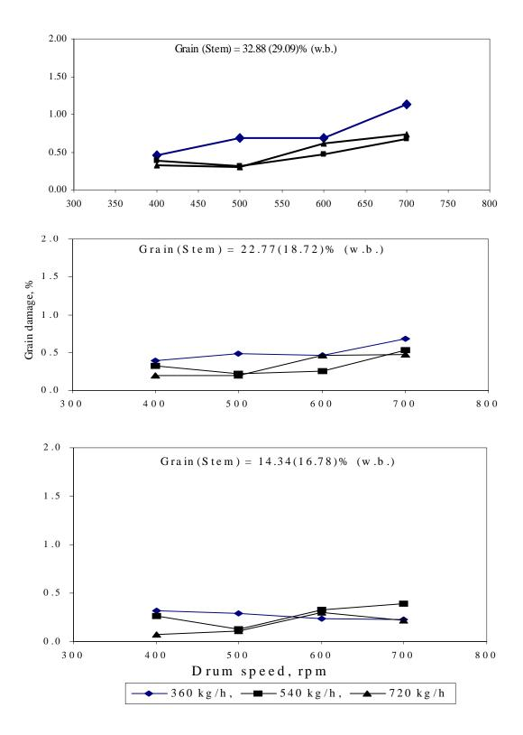
Figure 3: Effect of drum speed on grain damage at different grain moisture contents and feed rates.
