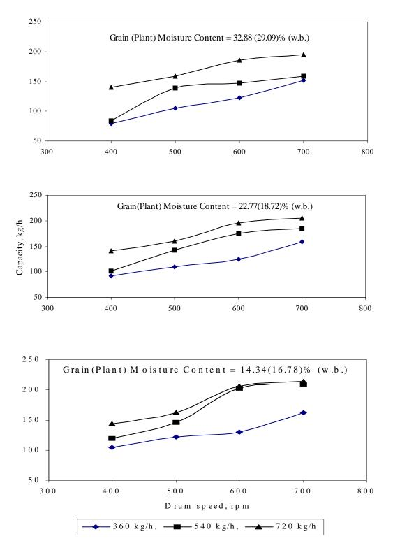
Figure 2: Effect of drum speed on capacity at different grain moisture contents and feed rates.
