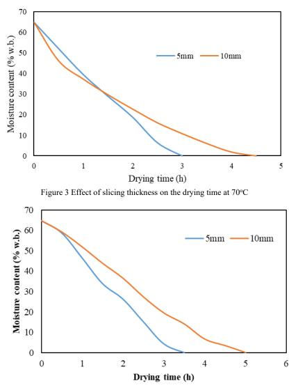
Figure 4 Effect of slicing thickness on the drying time at 60°C
