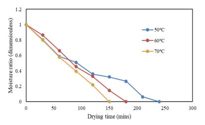
Figure 1 Drying curve of 5 mm thickness slices at various temperatures
