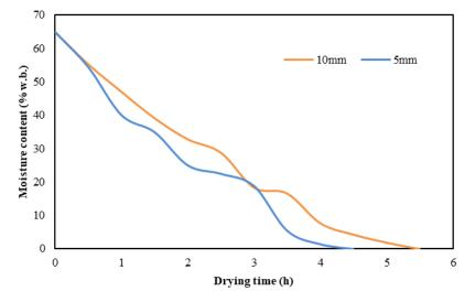
Figure 5 Effect of slicing thickness on the drying time at 50°C
