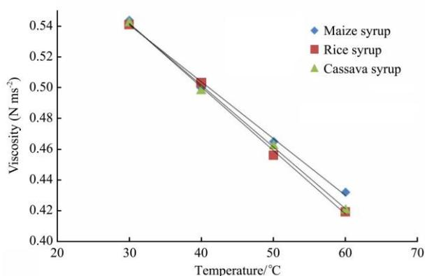
Figure 3 Effect of temperature on viscosity of the syrups
