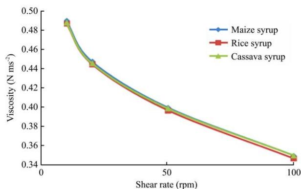
Figure 4 Effect of shear rate on viscosity of the syrups
