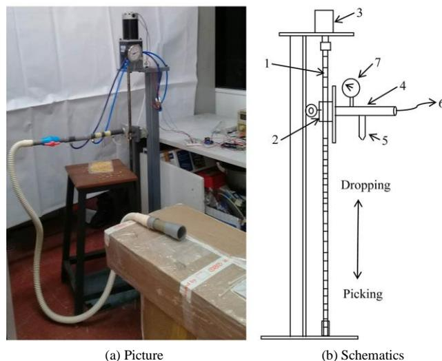
Figure 6 Nozzle performance test set up
