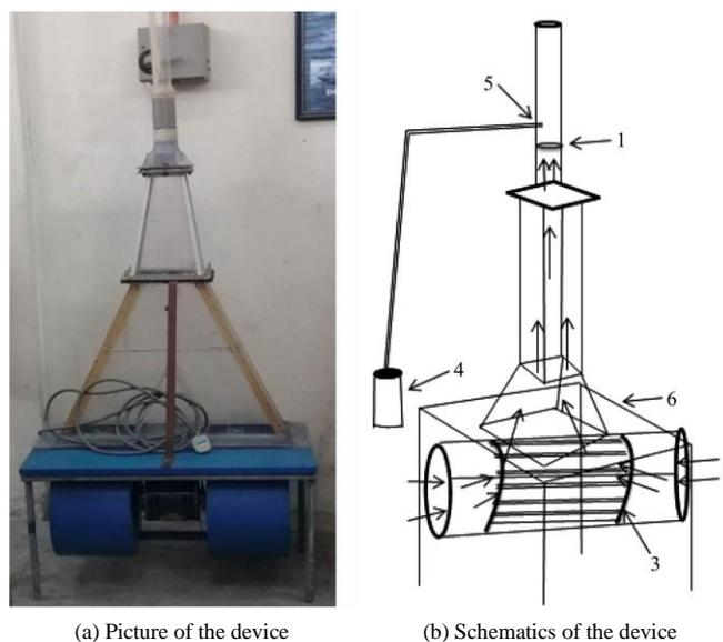
Figure 3 Terminal velocity measurement device
