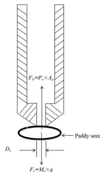
Figure 2 Seed- nozzle kinematics
