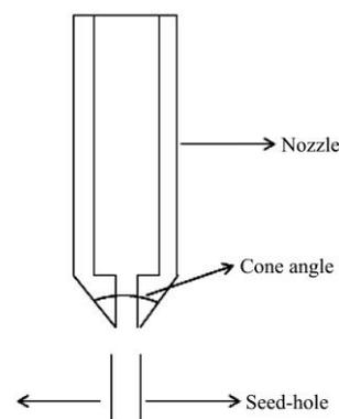
Figure 5 Cross section of seeding nozzle
