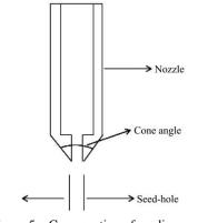
Figure 5 Cross section of seeding nozzle
