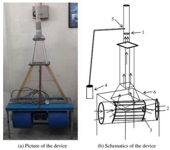
Figure 3 Terminal velocity measurement device
