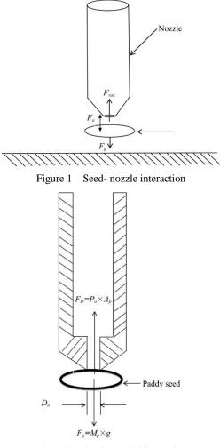
Figure 2 Seed- nozzle kinematics
