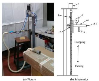
Figure 6 Nozzle performance test set up
