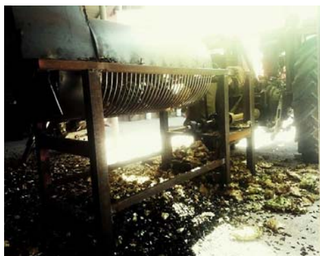
Figure 1 Fabricated sunflower threshing unit
