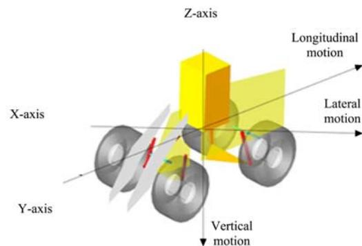
Figure 7 Tractor body-centered axis system
