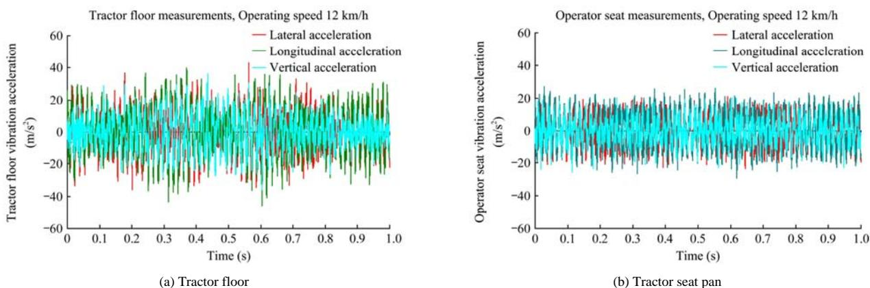
Figure 11 Time history of the raw signal-vibration acceleration
