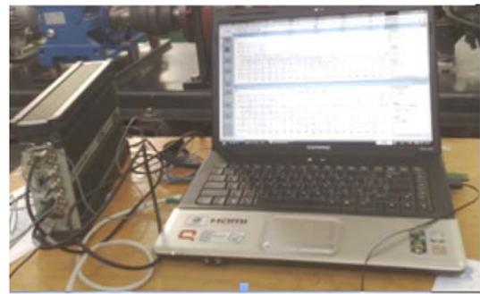
Figure 6 The vibration Measurement system
