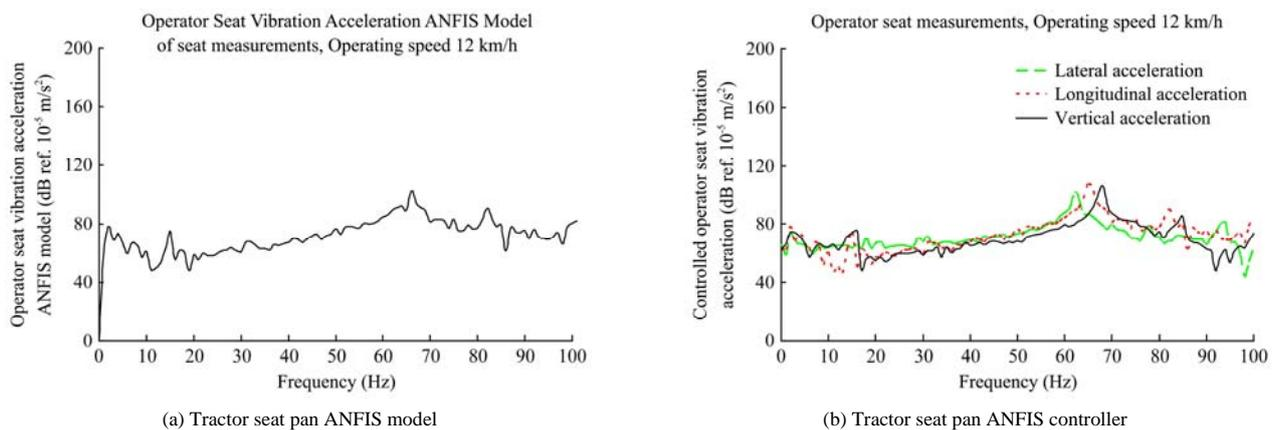
Figure 14 FFT of controlled vibration acceleration
