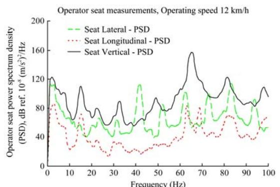
Figure 15 PSD for uncontrolled vibration accelerations measured in tractor seat pin
