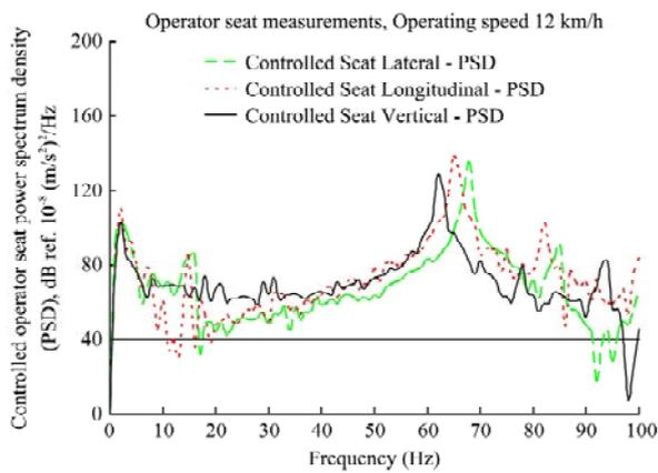
Figure 16 PSD for controlled vibration accelerations measured in tractor seat pin
