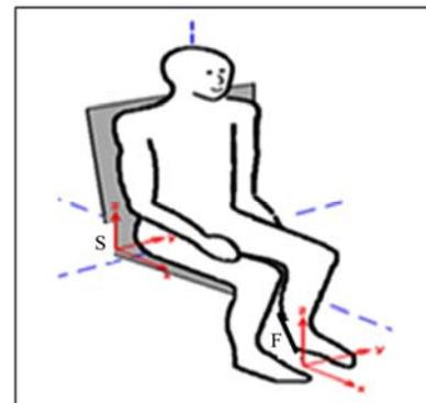
Figure 1 Direction of vibration measurements and location of accelerometers for a tractor
