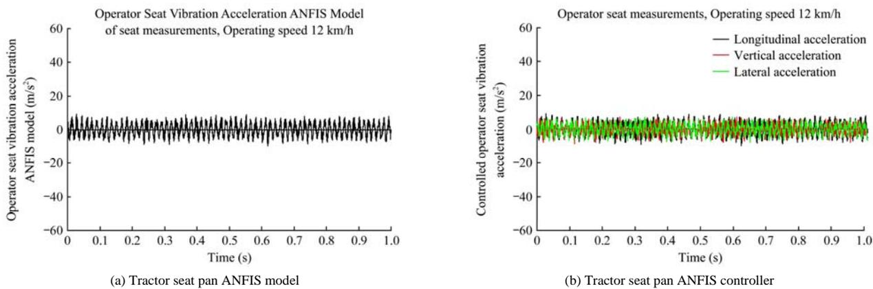
Figure 12 Time history of the controlled signal-vibration acceleration
