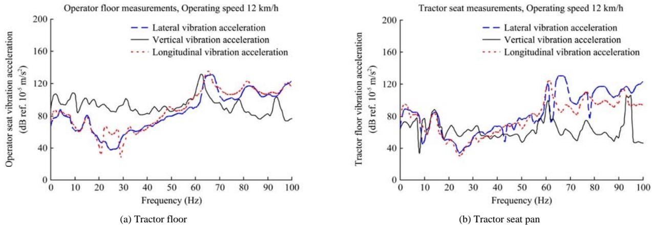
Figure 13 FFT of weighted vibration acceleration
