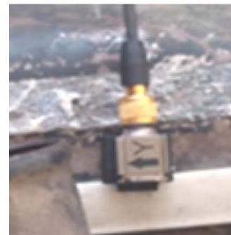
Figure 8 Tri-axis accelerometers
