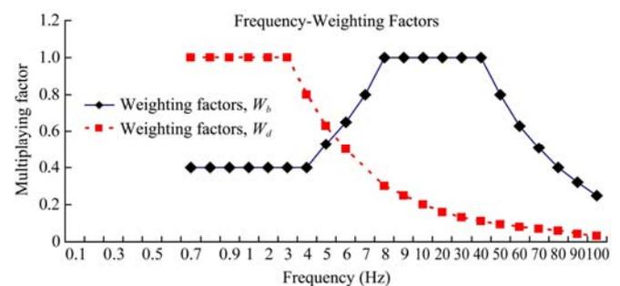
Figure 2 BS 8641 frequency weighting filter (Nahvi et al., 2009)
