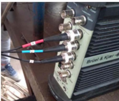
Figure 5 The PULSE for analysis system
