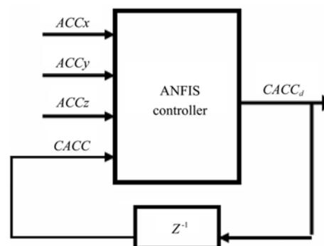
Figure 4 ANFIS controller for floor acceleration
