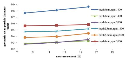
Figure 3 Effect of moisture content on geometric mean particle diameter
