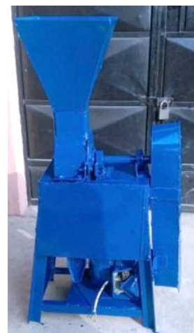
Figure 9 Fully developed almond seed extractor
