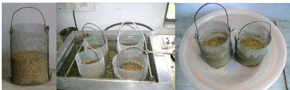
Figure 1 The laboratory arrangement for soaking experiments
