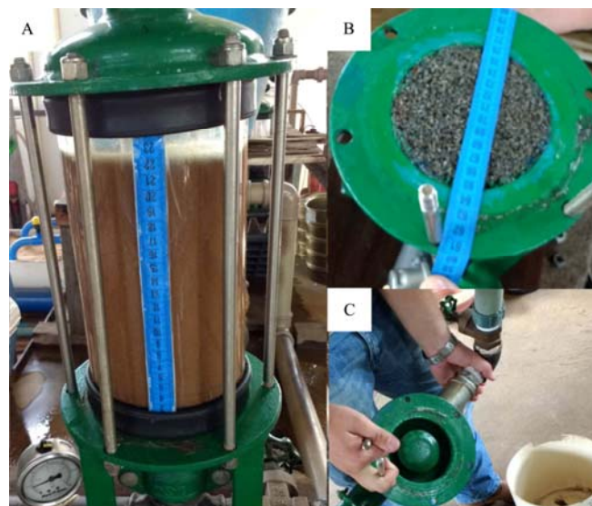
Figure 2 Sand filter prototype in operation, with details of the acrylic filter body (A), porous surface drainage system (B) and diffuser plate (C)
