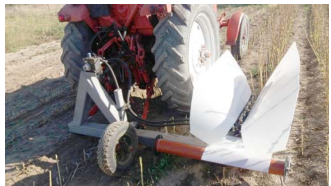
Figure 10 Photo of the one-row experimental device for feeding sesame stems
