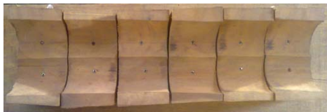
Figure 6 Female side of a mold for shaping the aluminium sheet into a CPC
