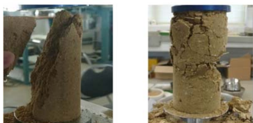
Figure 13 Failure mode of control sample (left) and soil-shell husk-cement (right)
