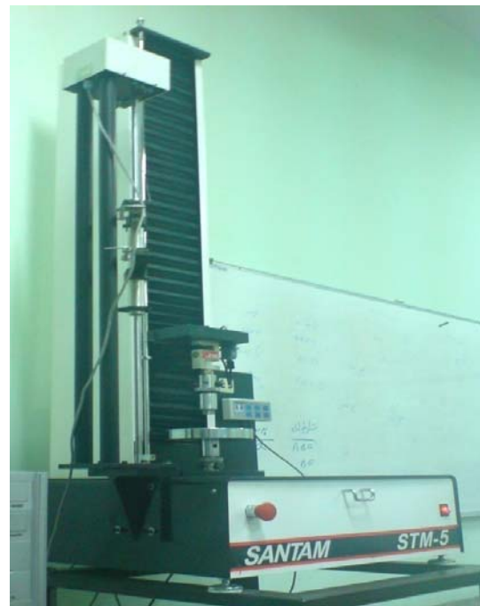
Figure 2 Tension/compression testing machine for the measurement the mechanical properties of chickpea stems (Instron Universal Testing Machine /SMT-5, SANTAM Company)
