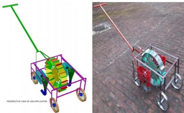
Figure 1 Isometric and photographic view of the applicator
