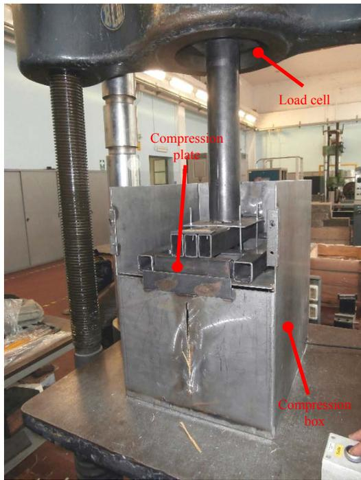
Figure 5 Straw mechanical characterisation setup
