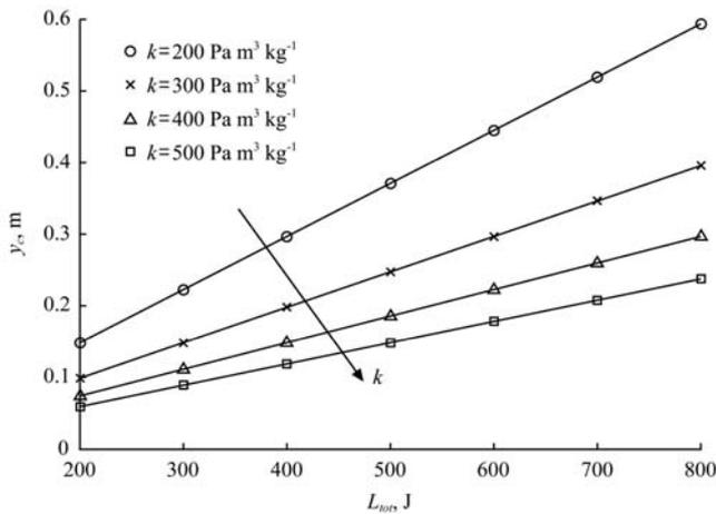
Figure 3 Piston stroke  $y_c$  per cycle related to the total work for each cycle  $L_{tot}$  (straw stiffness constant  $k$ ,  $m_{tot} = 17.5$  kg,  $\rho_s = 30$  kg  $m^{-3}$ ,  $\rho_f = 120$  kg  $m^{-3}$ )
