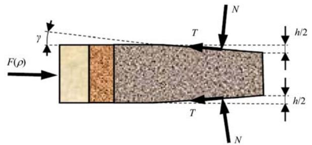
Figure 2 Mechanism to regulate the density of the bale
