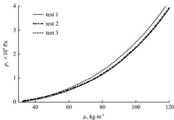
Figure 6 Straw mechanical characteristic
