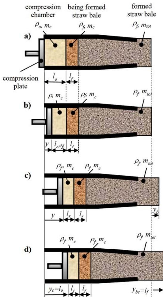
Figure 1 Schematic of the steps needed in a compression cycle with a continuous production of bales
