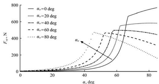
Figure 7 Operating force  $F_{op}$  versus the lever angle  $\alpha$ , for different initial values  $\alpha_o$
