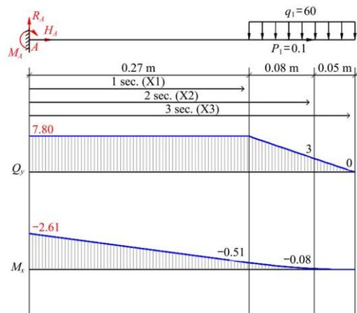
Figure 4 Shear force (*Q<sub>y</sub>*) and bending moment (*M<sub>x</sub>*) diagram of cultivator tyne considering, Cultivator tyne as a cantilever beam fixed at point A. Cultivator self-load, *P<sub>1</sub>*=0.1 kN and soil resistive force (*q<sub>1</sub>*) as a distributed load of 60 kN m<sup>-1</sup> on tyne
