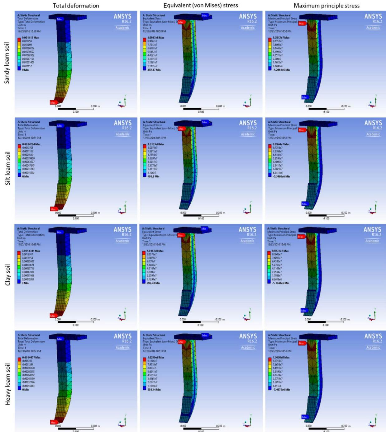
Figure 7 ANSYS simulation results of total deformation, equivalent (von Mises) stress, and maximum principle stress for sandy loam, silt loam, clay and heavy loam soil test cases. Each row represents results for each test case. Max and Min tags in each results showing maximum and minimum value of the output
