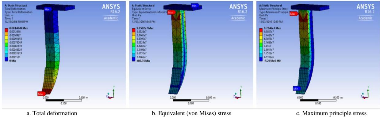
Figure 6 ANSYS simulation results for sandy soil case
