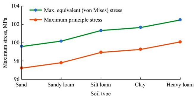
Figure 8 Maximum stress for different soil condition based on ANSYS simulation output
