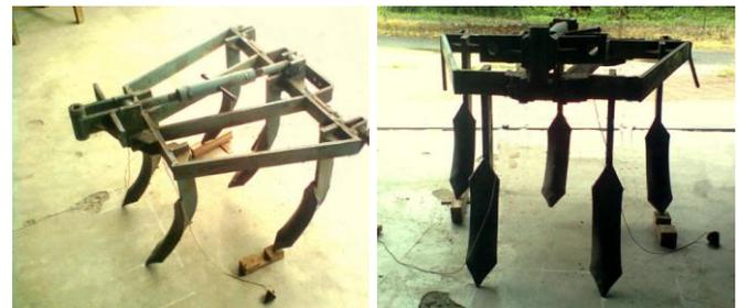
Figure 1 The 5-tyne cultivator prototype with isometric and front view
