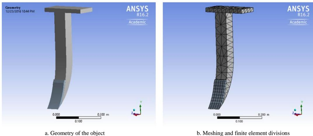
Figure 5 Cultivator tyne geometry
