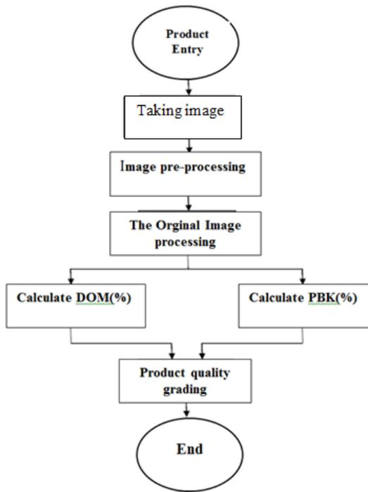
Figure 2 Major stages of program progress for the classification of rice using image processing
