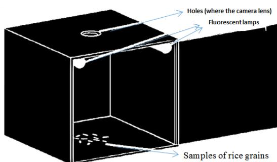
Figure 1 A schematic of the box used for imaging
