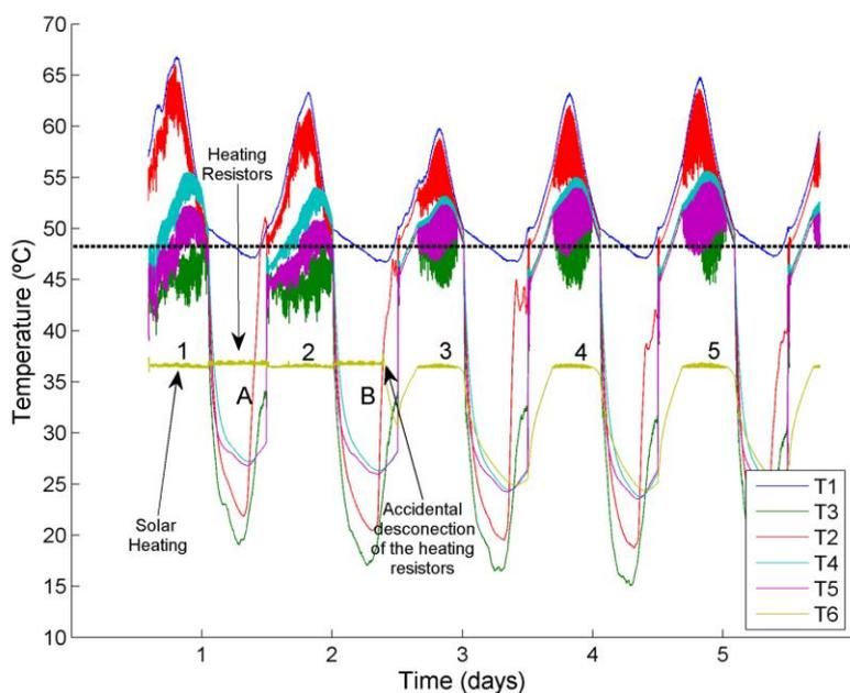
Figure 7 Experiment 2 temperatures on the solar circuit and inside the incubator. During the 2<sup>nd</sup> night (period B) the electrical power of the incubator was accidentally disconnected.
