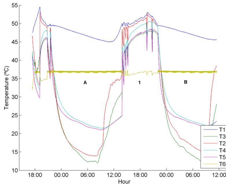
Figure 10 Experiment 3 temperatures. 'A' and 'B' are periods with electrical heating. During the 'A' period, there is solar heating.
