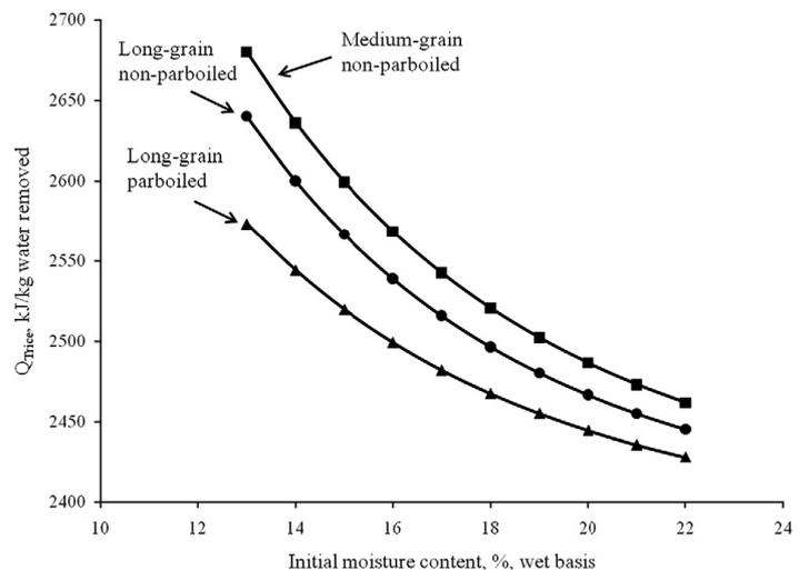
Figure 2 Energy required to dry rice ( $Q_{Trice}$ ) to 12.5% (wb) moisture content for long-grain non-parboiled, long-grain parboiled and medium-grain non-parboiled rice at 60 °C. (Billiris et al., 2011)
