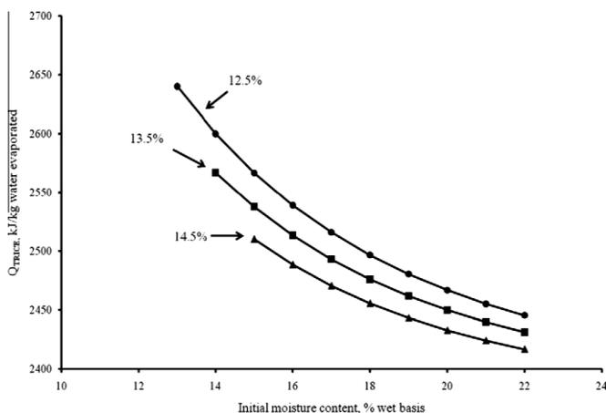
Figure 1 Total energy required to dry rice ( $Q_T$ ) to 12.5%, 13.5%, and 14.5% (wb) moisture content of the long-grain, non-parboiled rice at 60 °C. (Billiris et al., 2011)
