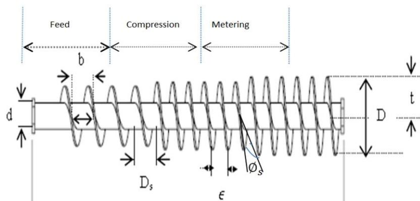
Figure 1 Auger Geometry [ $D$  = barrel diameter (mm),  $D_s$  = distance between axis of flight screws (mm),  $d$  = shaft diameter (mm),  $t$  = pitch length (mm),  $b$  = channel width (mm),  $\epsilon$  = pitch of helix (mm),  $\phi_s$  = helix angle (deg.)].
