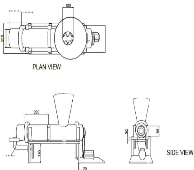
Figure 4 Projection (third angle) of the single screw extruder
