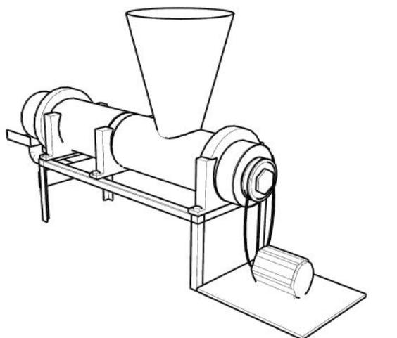
Figure 3 Isometric drawing of the single screw extruder
