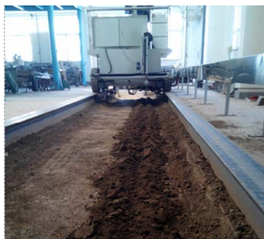
b. Soil surface condition after subsoiling
