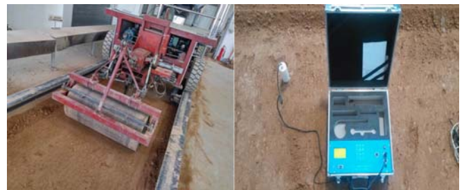
Figure 4 Soil preparation unit (left) and soil parameters measurement device (right) in soil bin
