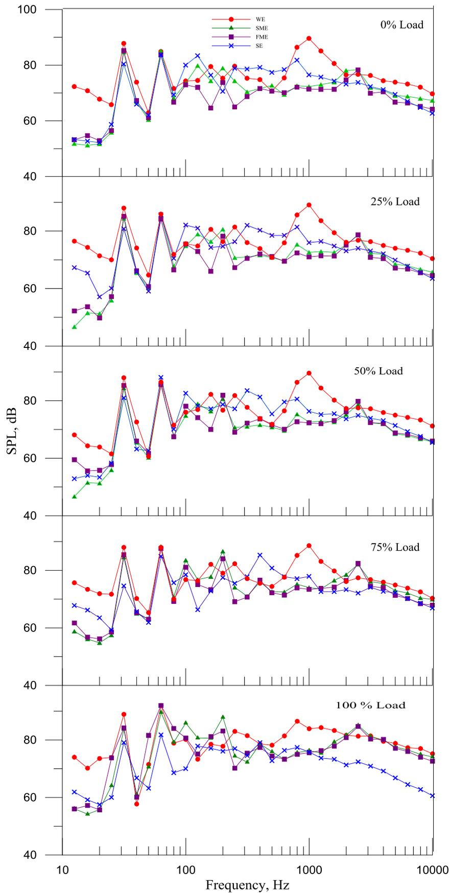
Figure 8 The 1/3<sup>rd</sup> octave sound pressure levels (SPL) of the generator for different conditions at (a) no load, (b) 25% load, (c) 50% load, (d) 75% load, and (e) full load
