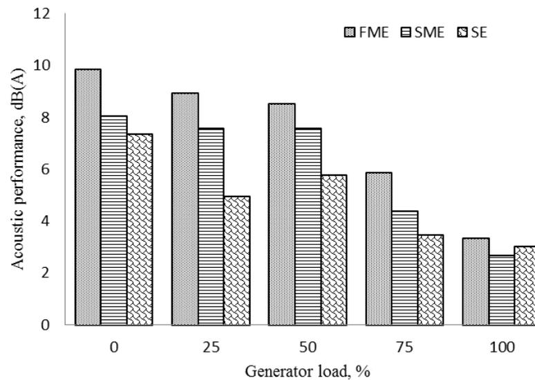
Figure 10 The acoustic performance of different enclosures at different generator loading conditions
