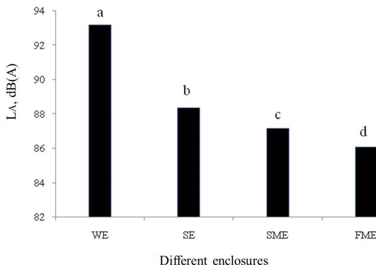
Figure 11 The effect of different enclosure setups on the A-weighted generator sound
