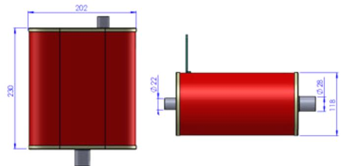
Figure 1 The generator engine reactive muffler dimensions, mm
