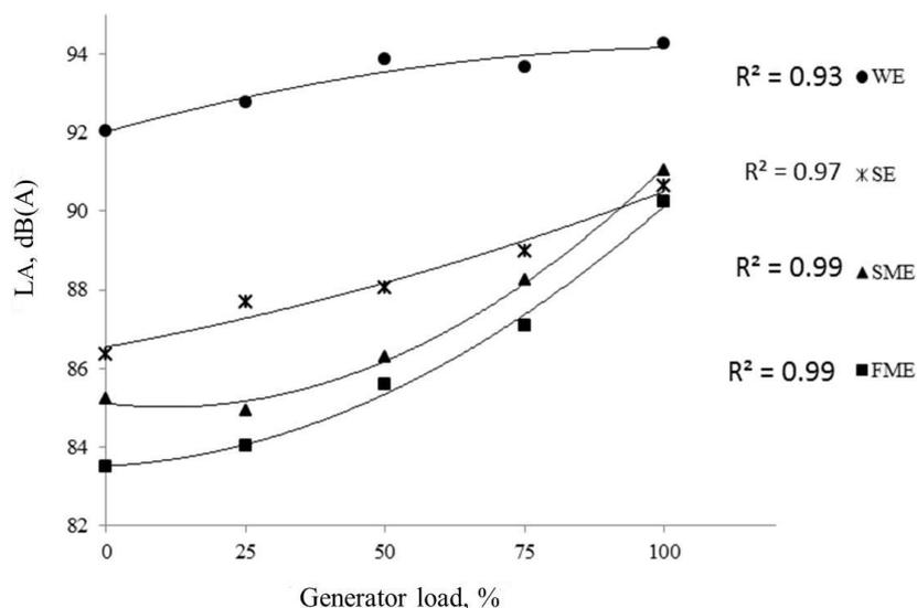
Figure 9 The overall generator sound for different setups at varying generator loading conditions
