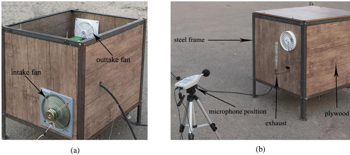
Figure 2 The developed simple enclosure (a) without upper panel and (b) complete
