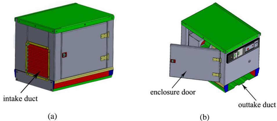
Figure 3 The developed modified enclosure (a) closed door (fully covered modified enclosure, FME) and (b) open door (semi covered modified enclosure, SME)
