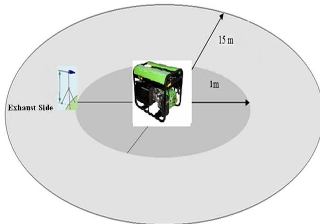
Figure 5 The schematic diagram of the sound measurement test site
