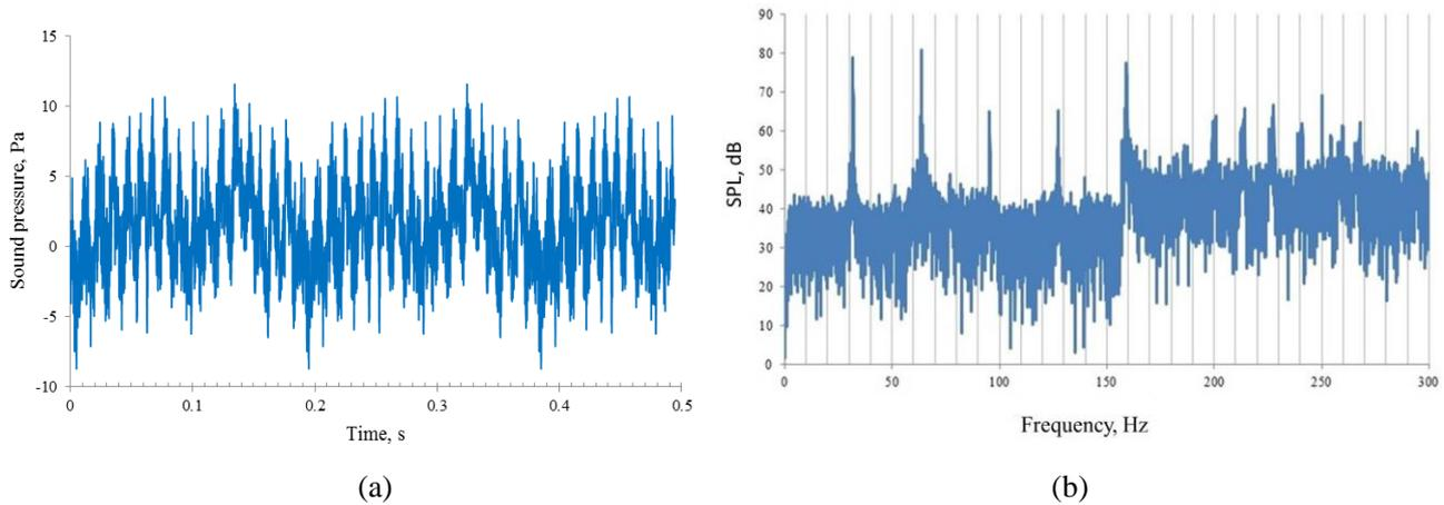
Figure 7 The sound signal for fully covered generator by modified enclosure in front of the generator exhaust at full load condition: (a) The time history and (b) Narrow band frequency domain signal
