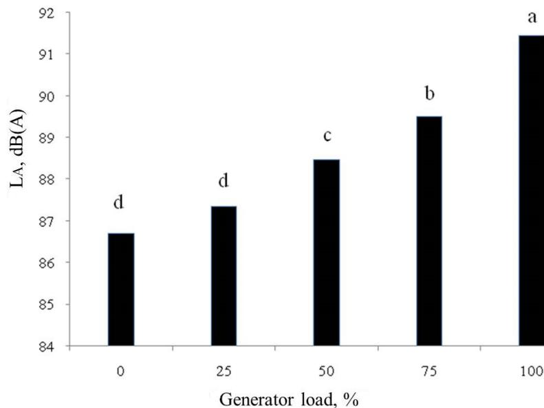
Figure 12 The effect of generator loading conditions on its A-weighted sound
