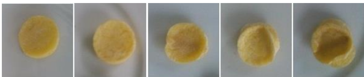
Figure 7 Change in size of potato slices as drying proceeded (at section two-four)
