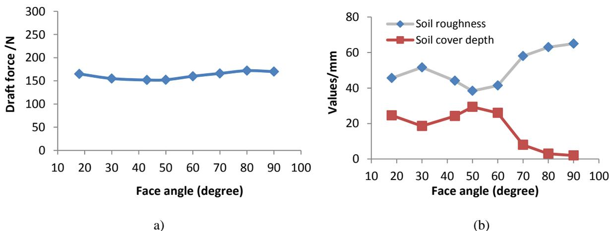
Figure 9 Simulation results for different face angles of the paired-row opener at a constant wing angle of 18 °
