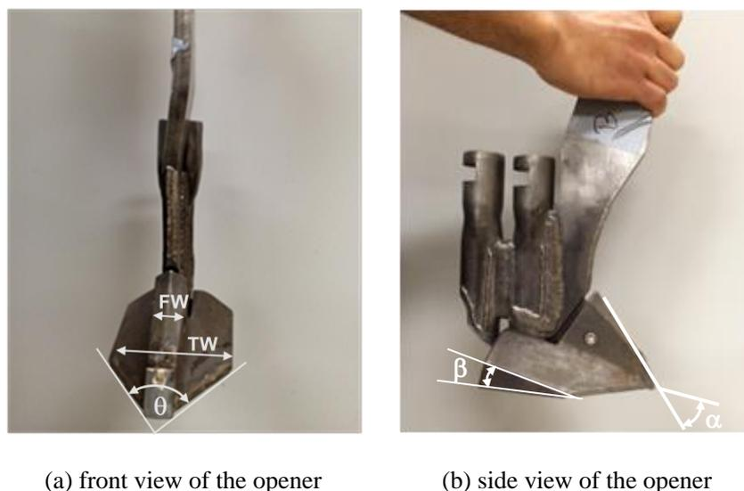
Figure 1 The paired-row opener tested;  $\alpha$  = face angle;  $\beta$  = wing angle;  $\theta$  = sweep angle; FW = face width; TW = tool width
