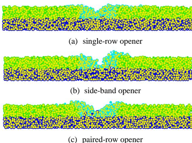
Figure 6 Screenshots of soil cross-sections from simulations of different types of openers; colours show different soil layers and the centre zone of the tool path
