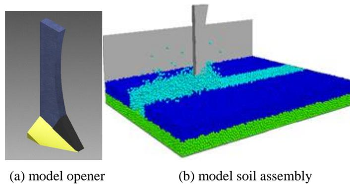
Figure 3 Soil-opener model; y is the opener travel direction
