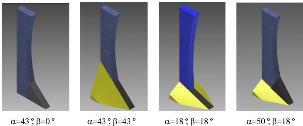
Figure 5 Examples of model openers simulated;  $\alpha$  and  $\beta$  stand for face and wing angles respectively;  $y$  is the opener travel direction
