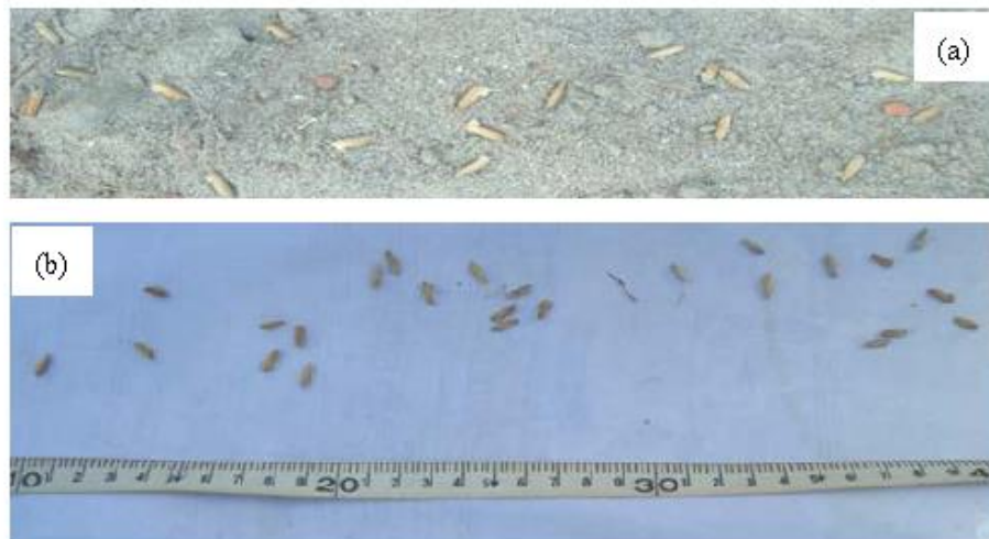
Figure 12 (a) Distribution pattern of seed on dry land, (b) Distribution pattern of seed on white paper
