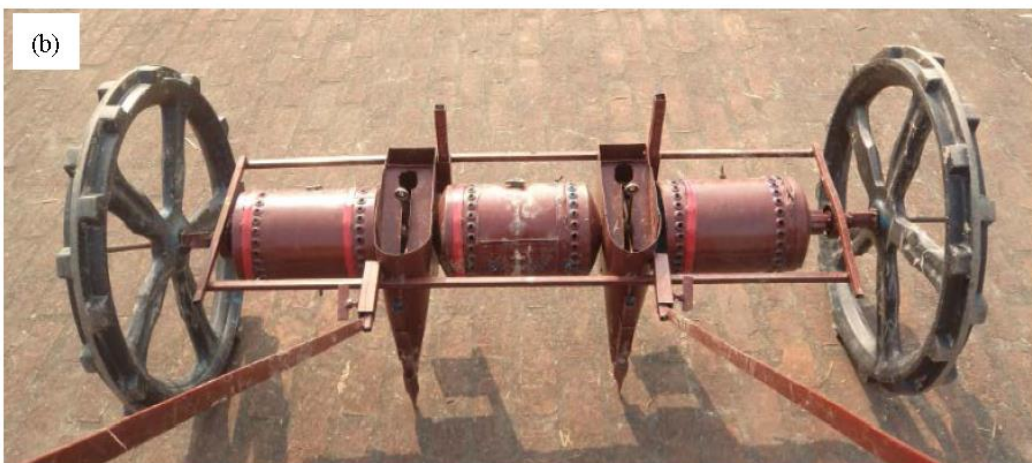
Figure 7 (a) Different schematic views of drum seeder with urea supergranule application, (b) Photographic view of drum seeder with urea supergranule application
