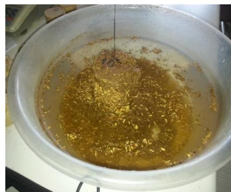
Figure 7 View of pepper crop briquette after water resistance test
