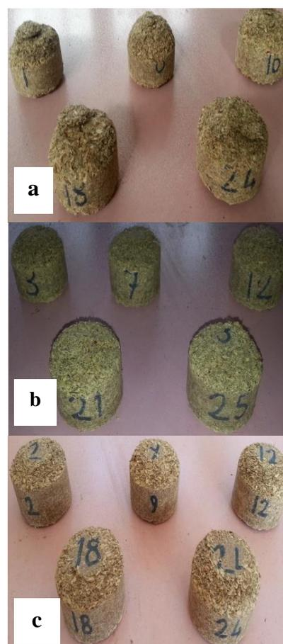
Figure 5 Views after tumbler testing briquettes produced at 115 MPa (a), 150 MPa (b) and 185 MPa (c) compaction pressure
