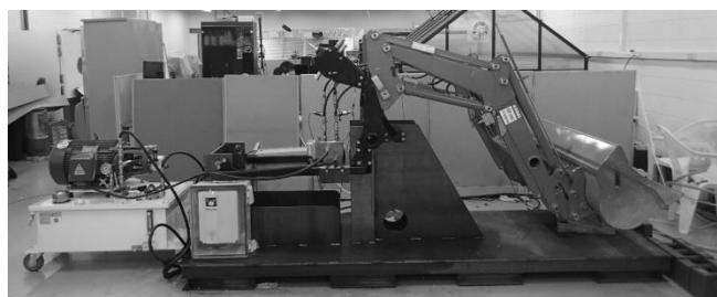
Figure 1 Simulator of a front-end loader control system connected with an EHPV
