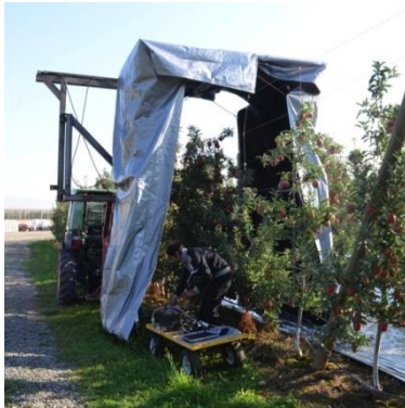
Figure 1 Over the row sensor platform used to acquire images of apple trees in commercial orchards in Grandview, WA and Prosser, WA (Gongal et al., 2014)
