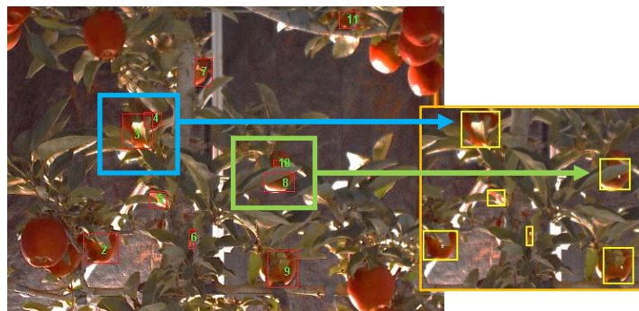
Figure 6 Fragments of the same apple merged together using a clustering method as represented by smaller boxes in the right image.
