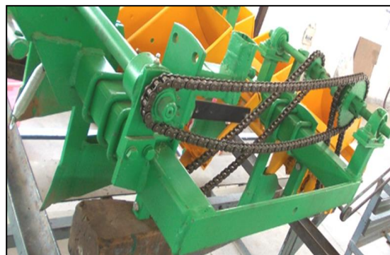
Figure 4 Power transmission system of the machine
