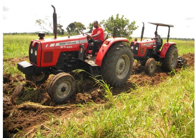
Figure 2 A photograph depicting tractor- dynamometer, implement mounted position during disc ploughing operations
