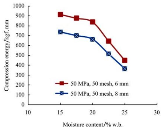
Figure 3 Effect of mold diameter and moisture on compression energy
