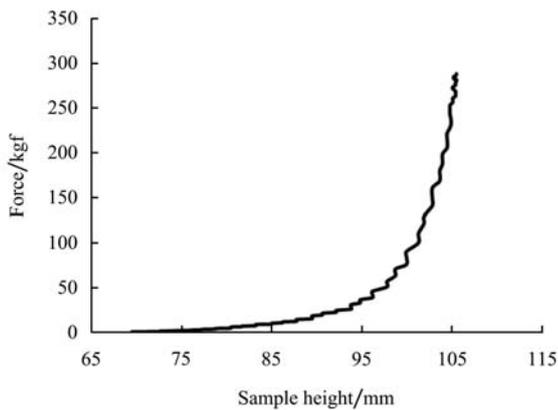
Figure 1 Compression energy in maximum pressure of 100 Pa, moisture 15% and size 30
