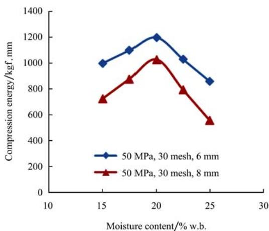
Figure 2 Effect of mold diameter and moisture on energy consumption for compression
