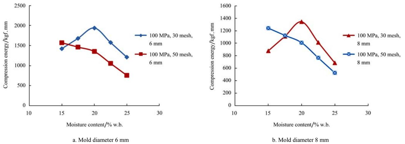
Figure 7 Effect of particle size and moisture on energy consumption
