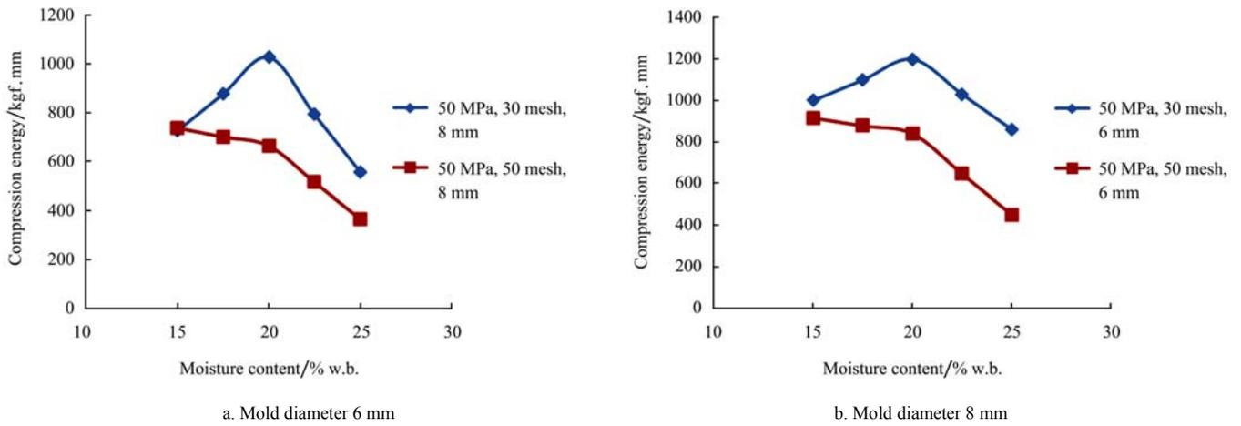
Figure 6 Effect of particle size and moisture on energy consumption
