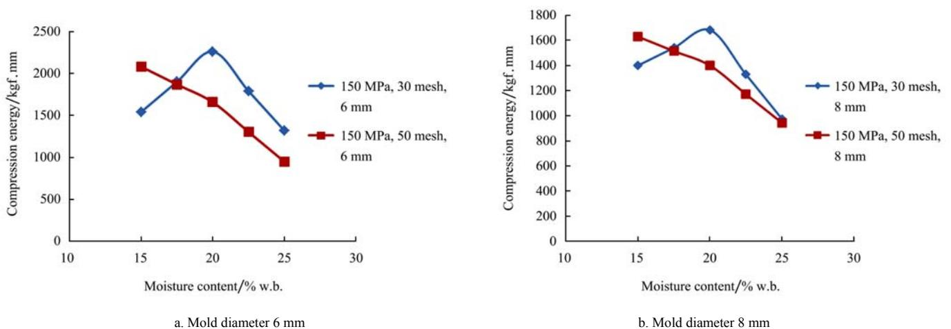
Figure 8 Effect of particle size and moisture on energy consumption
