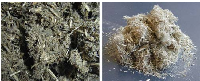
Figure 2 Wet extruder fibre material (left) and dried fibre material after milling in extruder and disc mill (right)
