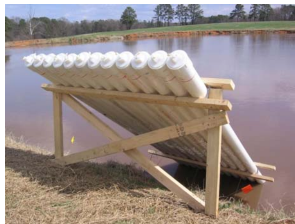
Figure 1 Placement of the experimental units (EUs) in the lagoon. The EUs are capped at the top with a threaded PVC connector glued to the pipe.
