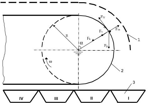
Figure 1. The scheme of transporter type electric separator: 1-potencial electrode; 2- grounded electrode; 3-classifier pans
