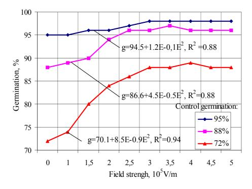
Figure 2. The relationship between the seeds germination and the strength of electric field
